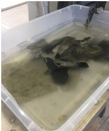
Figure 4: Shallow rinsing tray use for sample clean up
